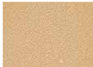
Standard powder paint with degassing additive, mixed by hand, magnified 6.5 times
