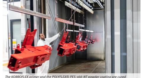
The KORROFLEX primer and the POLYFLEX® PES-166-NT powder coating are cured in two ovens at 190–200°C for a maximum of 30 minutes.
