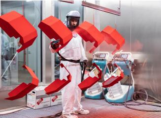
The primer and the top coat are applied manually in a walk-in booth.
