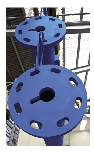
The low temperature powder coating is characterized by smooth design and uniform coating thickness.
