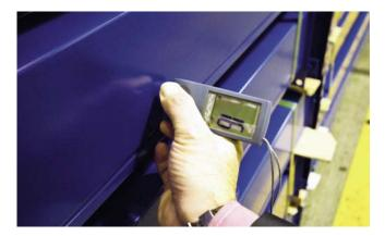
With ultra thin layer NT powder coating one can obtain a high covering power and smooth surfaces with 16 µm layer thickness.
