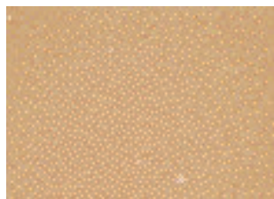
Standard powder coating with degassing additive, mixed by hand, magnified 6.5 times
